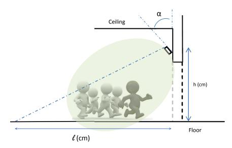
Size of the detection area according to the tags used for  $h = 250 \text{ cm}^{(1)}$
